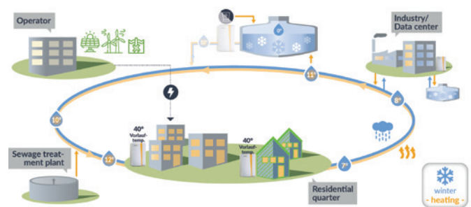
Exemplary illustration of a low temperature heat grid and its participants
